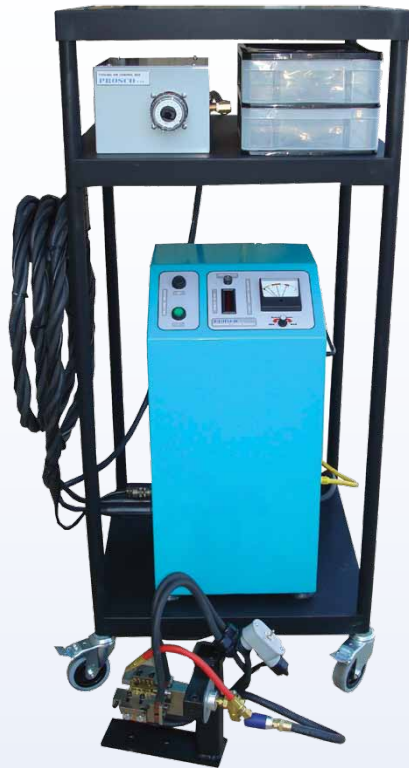
Main Power Supply Unit, Power Cables, Adjustable Tool Holder, and Custom-Designed Tool Post
