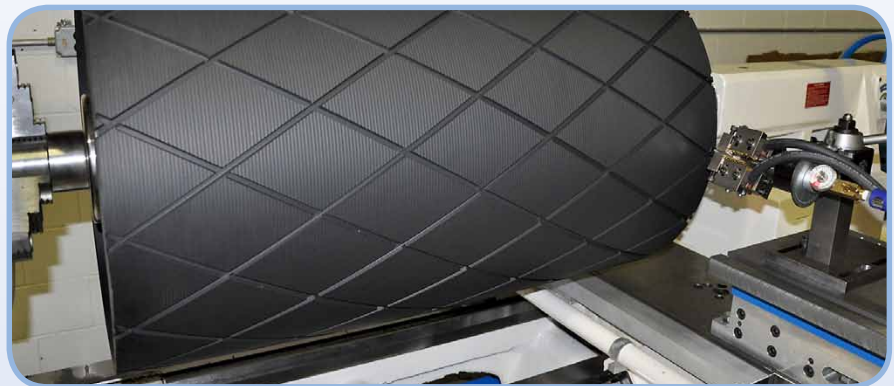
Various types of clean grooves can be produced efficiently
